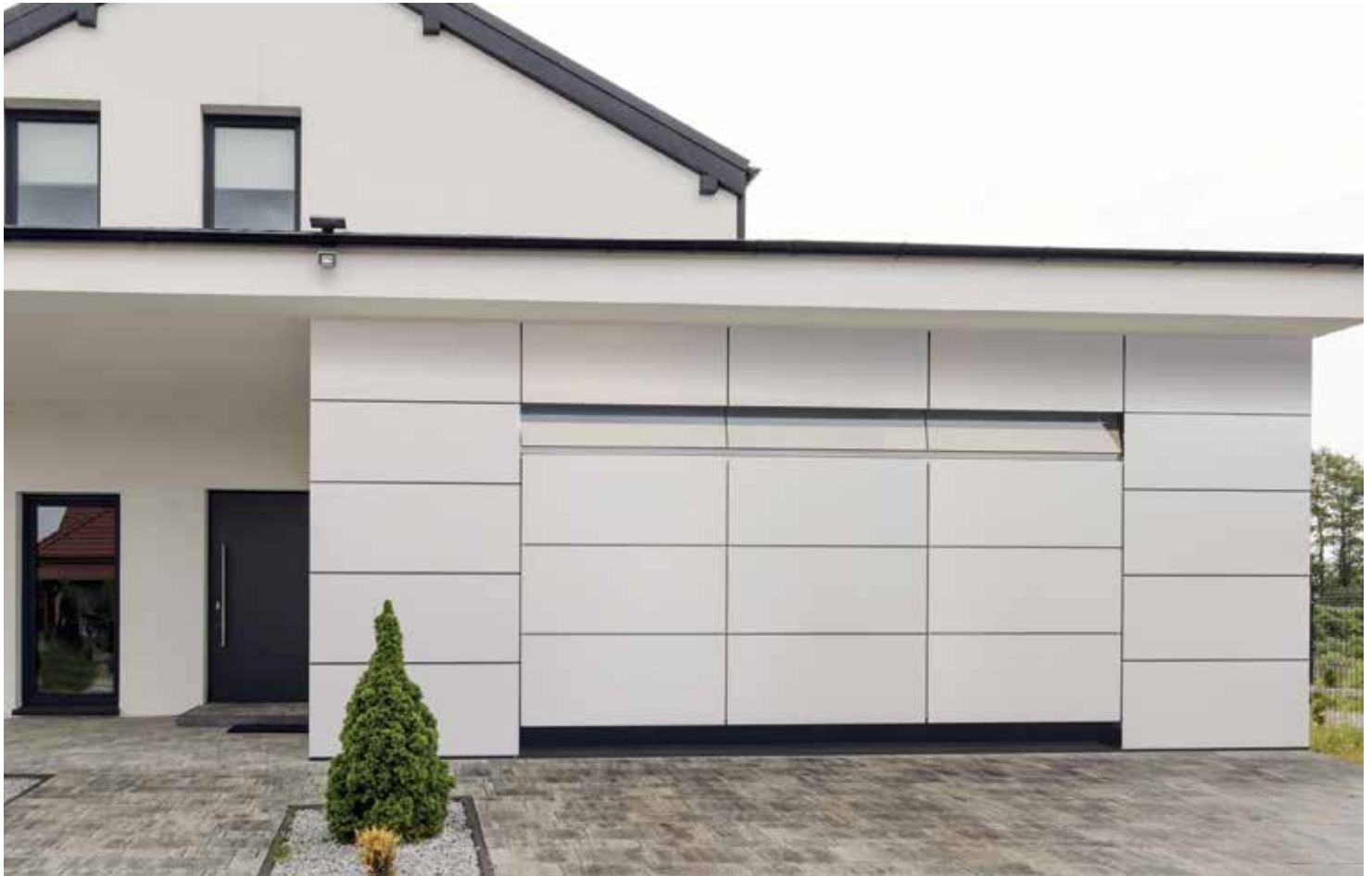
Facade flush sectional doors give a possibility to conceal garage doors.
